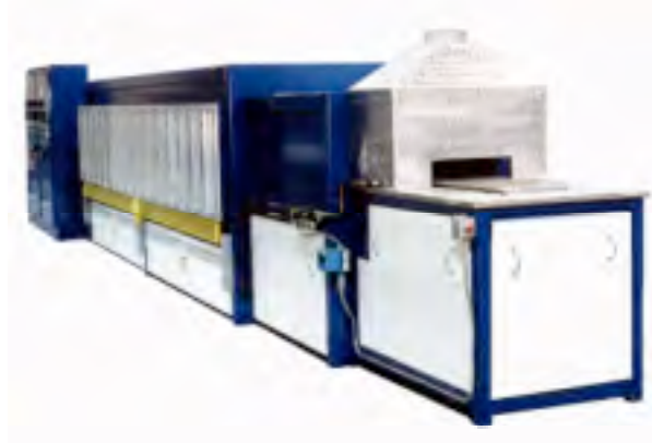
Figure 1. Controlled Atmosphere Brazing Furnace.
