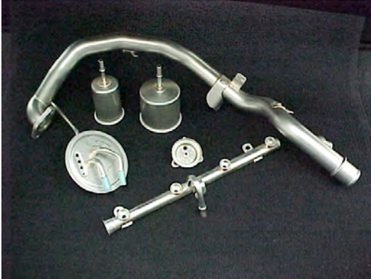
Figure 1. Brazed Stainless Steel Components
